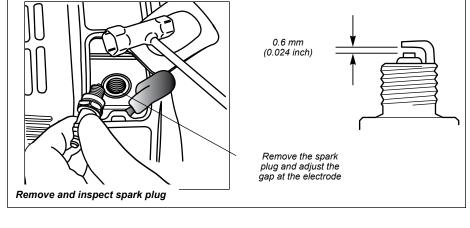
■ Replace the spark plug annually: Use only NGK CMR5H or equivalent resistor type spark plug of the correct heat range. Set spark plug electrode gap to 0.6 mm (0.024 inch).
